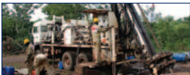
Foremi diamond core rig in operation at Tongon.
