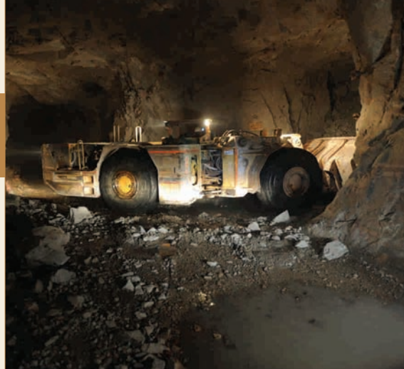
CAT1700 underground loader in the first longhaul stope at Yalea.
